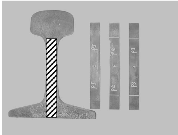
Figure 1 Rail web test specimens.
